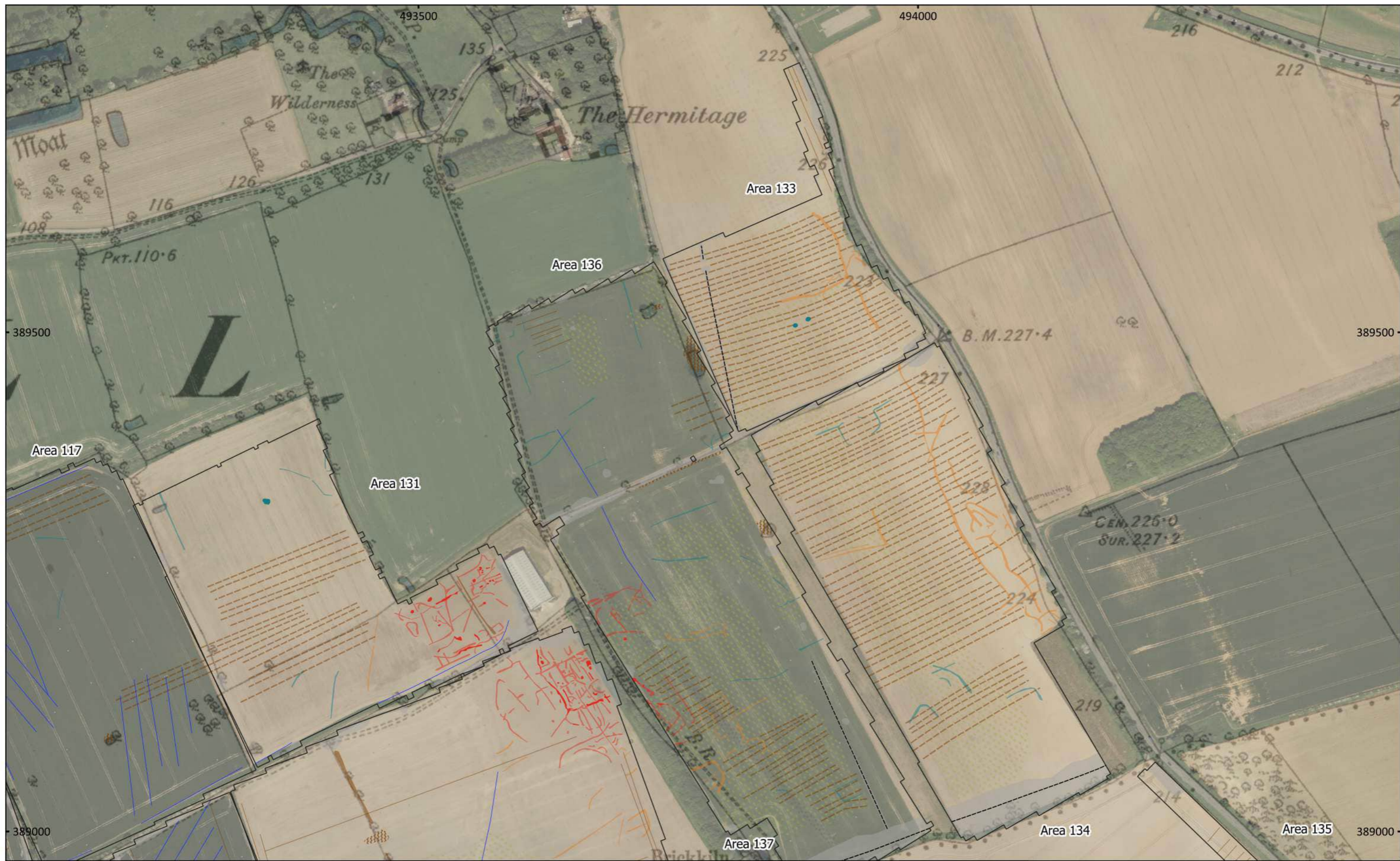
MSSK1393: Tillbridge Solar Scheme, Lincolnshire Figure 27 - Magnetic Interpretation Over Historical Maps (Overview) (Eastern Areas 117-118 and 131-137) 1:3,500 @ A3 Copyright Magnitude Surveys Ltd 2023 Contains historical mapping © CLS Data 2023: Ordnance Survey, 6" 2nd edition c. 1882-1913
