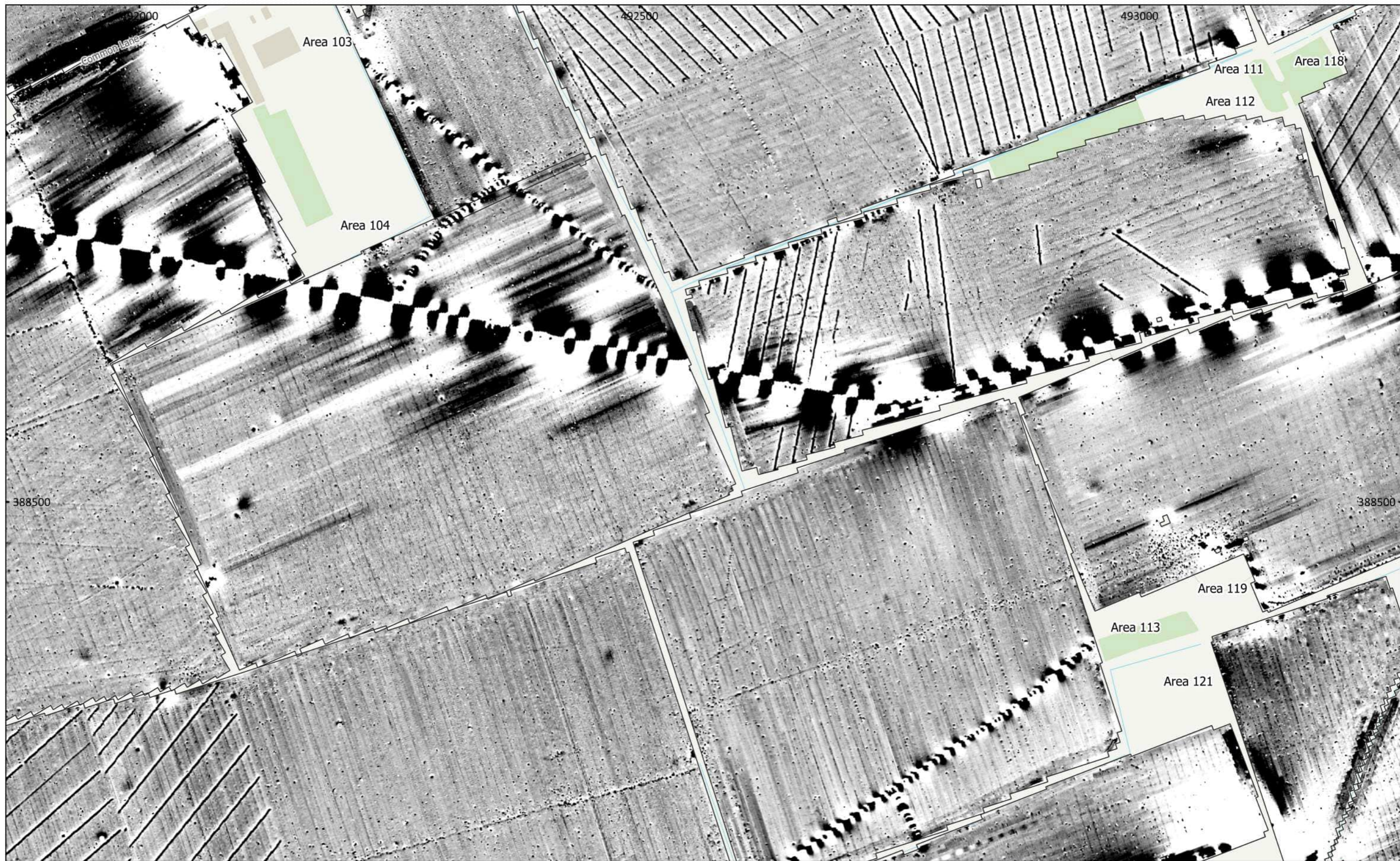
MSSK1393: Tillbridge Solar Scheme, Lincolnshire Figure 48 - Magnetic Total Field (Lower Sensor) (Overview) (Eastern Areas 90-91, 103-104, 112-114 and 119-121) 1:3,500 @ A3 Copyright Magnitude Surveys Ltd 2023 Contains Ordnance Survey data © Crown Copyright and database right 2023
