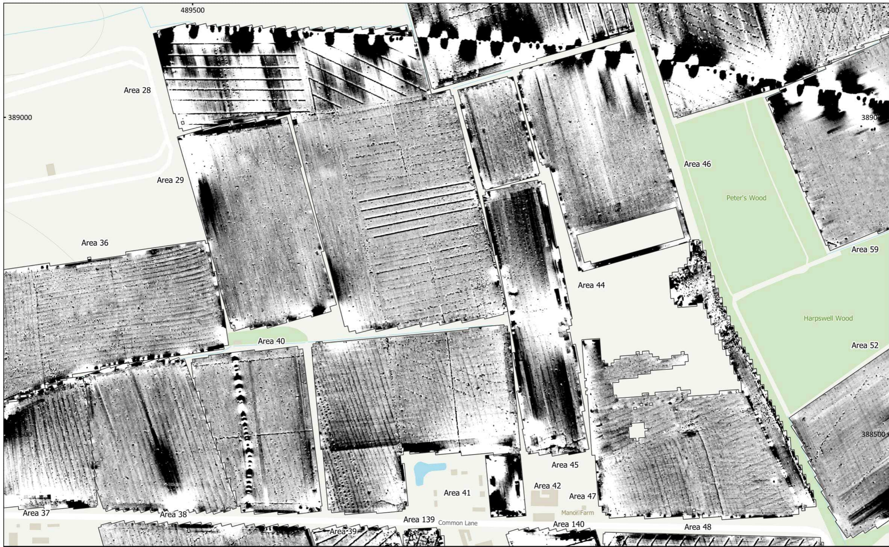
MSSK1393: Tillbridge Solar Scheme, Lincolnshire Figure 40 - Magnetic Total Field (Lower Sensor) (Overview) (South-Western Areas 29, 36-47 and 51-52 and 59) 1:3,500 @ A3 Copyright Magnitude Surveys Ltd 2023 Contains Ordnance Survey data © Crown Copyright and database right 2023
